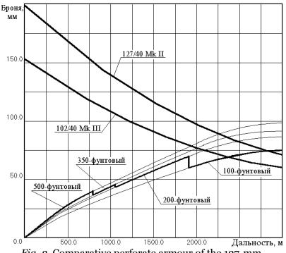
*Fig. 3.* Comparative perforate armour of the 127-mm, 102-mm shells and hypothetical armour piercing shell of a pneumatic gun
