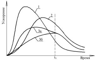
*Fig 2*. Projectile acceleration in the gun
