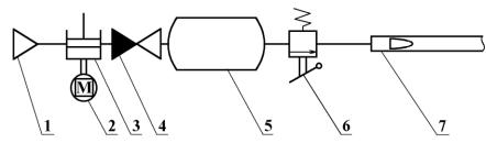
*Fig. 1.* The principal gun's pneuma-schematic: 1 - collector; 2 - compressor's drive; 3 - compressor; 4 - return valve; 5 - gas-reservoir; 6 - main valve; 7 – gun tube
