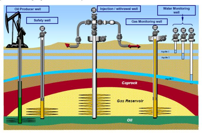
Fig 2: Basic elements of underground gas storage reservoir (Rodriguez et al., 2006).
