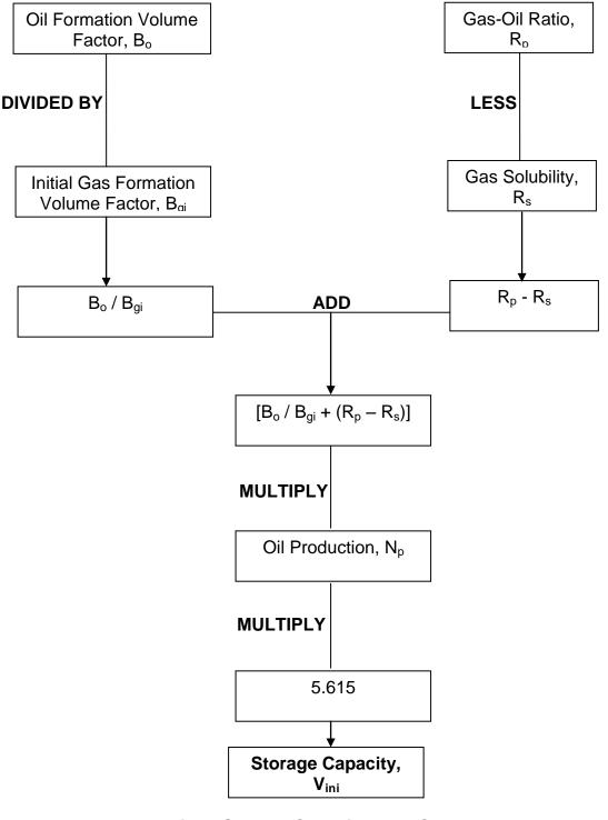
Fig 3: Storage Capacity Flow Chart
