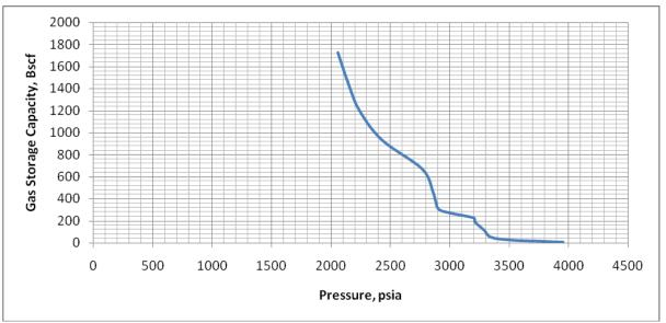
Fig 3.3: A plot of volume of gas to be injected at various pressures for reservoir Y-19.
