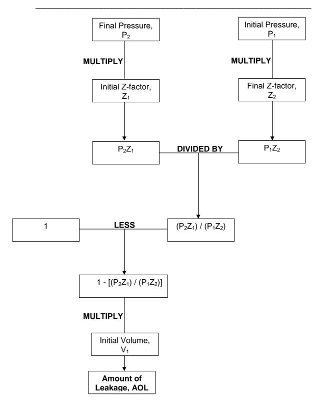
Fig 4: Flow Chart for Amount of Leakage from the Storage Reservoir
