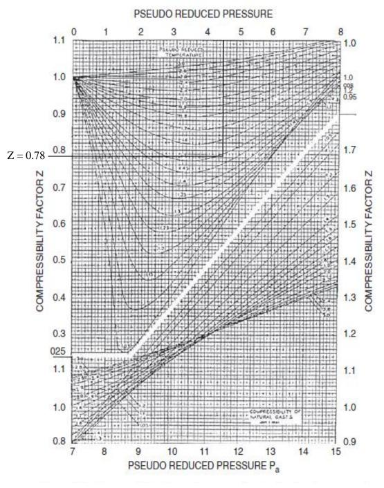
Fig 3.1: Compressibility of natural gas as a function of reduced temperature and pressure, Standing and Katz, (1942)
