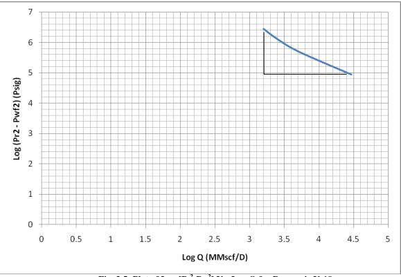
Fig. 3.5: Plot of Log [P<sub>r</sub><sup>2</sup>-P<sub>wf</sub><sup>2</sup>] Vs. Log Q for Reservoir Y-19
