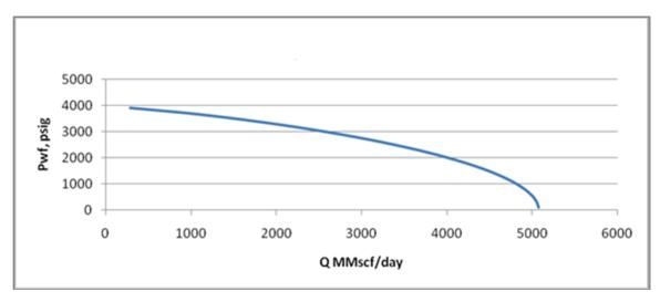
Fig. 3.7: A Plot of Well Flowing Pressure versus Deliverability, Y-19
