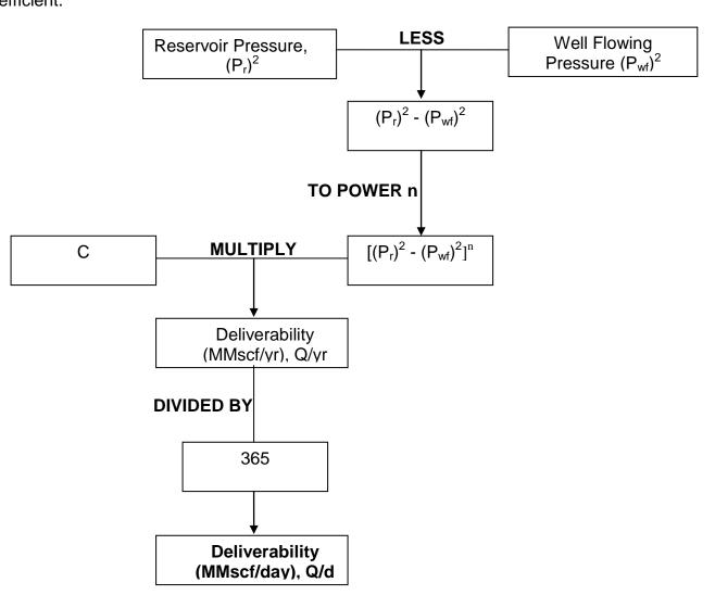
Fig 2.5: Flow Chart for the Deliverability of the Storage Reservoir
