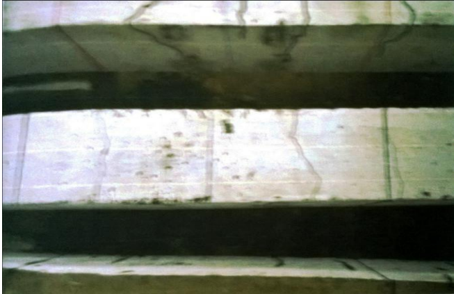
Fig 3 Beams failed upto 85% of the ultimate load of Flexural Deficient Control Beam (FDCB)
