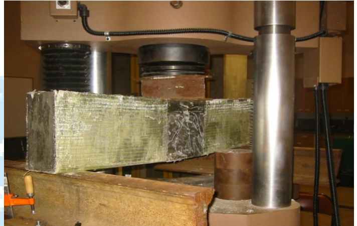
Fig 3 Beams failed upto 85% of the ultimate load of Flexural Deficient Control Beam (FDCB)
