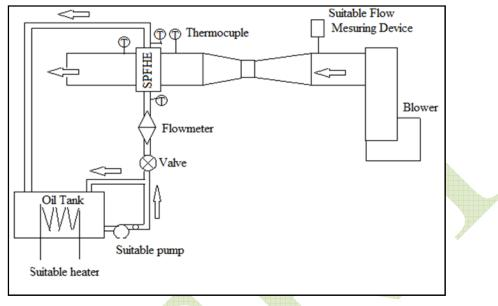
Fig. 3 Proposed experimental setup
