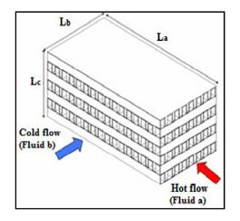
Fig. 2 Serrated Plate Fin Heat Exchanger (SPFHE) - For Air-Oil Cross Flow
