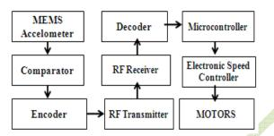
Fig1.system block diagram
