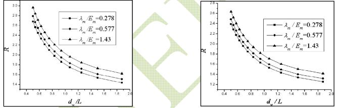
Fig. 8 Variation in R with dw/L for bolt size M20 (UDA) Fig. 9 Variation in R with dw/L for bolt size M20 (UPA)
