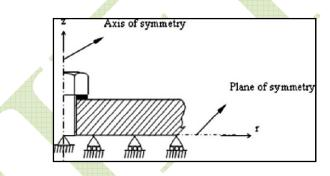
Fig. 4 Axisymmetric half model of the bolted joint
