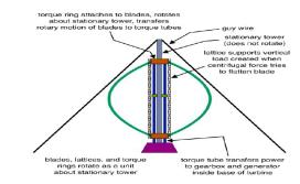
Figure 4: High Mechanical Efficiency Centrifugally Stable Darrieus Turbine
