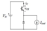
Fig. 2.1. The basic step down converter used in the analysis.
