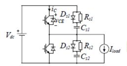
Fig. 3.3 a half bridge with one RCD snubber connected across each transistor.
