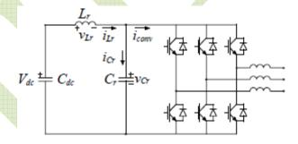
Fig. 4.1 The basic three phase resonant DC link converter.
