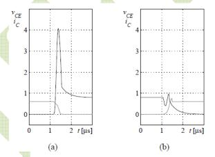
Fig. 3.3 Transistor collector current (black) and collector-emitter voltage (grey) at (a) turn-on and (b) turn-off of the upper IGBT in the converter consisting of a bridge leg. One RCD snubber is used across each IGBT. Note the high collector current peak at turn-on. Also note the poor behavior at turn-off.
