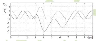
Fig. 4.2 Normalized inductor current (black) and resonant link voltage (grey) for a resonant DC link converter. The current fed to the converter is also shown (dashed). Note the resonant link voltage peak resulting from a decrease of the converter current.
