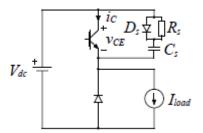
Fig. 3.1. The step down converter with the RCD snubber connected across the device output terminals.
