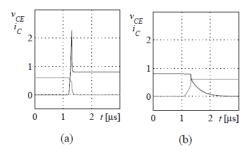
Fig. 2.2 Normalized transistor current (black) and voltage (grey) at (a) turn-on and (b) turn-off of the power transistor in the step down converter.
