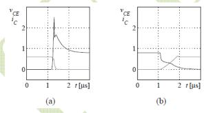
Fig 3.2 Transistor current (black) and voltage (grey) at (a) turn on and (b) turn-off of the power transistor in the step down converter with a full RCD charge-discharge snubber across the power transistor.
