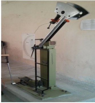
Fig. 8 Impact Testing Machine & its Specifications
