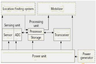
Figure 3. Components of a Sensor Node
