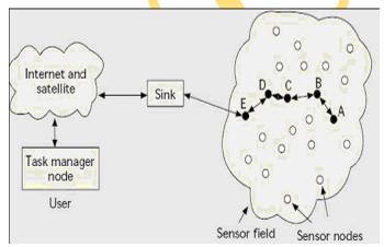
Figure: Basic Architecture of Wireless Sensor Network.
