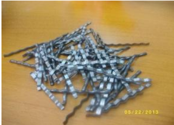
Fig 5. Steel fibers used for the production of FRSCC (a):LS, (b):HS.
