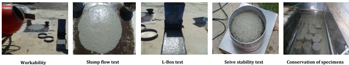
Fig 6. Workability tests on SCC.
