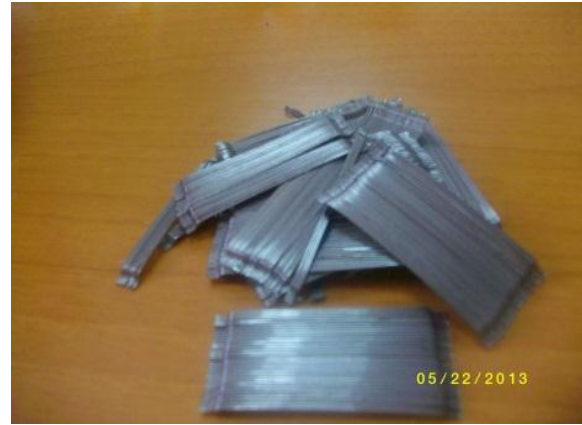
Fig 5. Steel fibers used for the production of FRSCC (a):LS, (b):HS.
