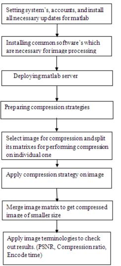
Fig. 5 Flowchart for implementation of compressing image in matlab Environment
