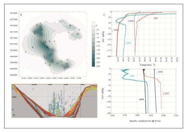
Figure 4. a. Bathymetric map of Rinjani Volcanic Lake (Segara Anak); b.  $CO_2$  bubbles in Segara Anak Lake were recorded by echo sounding; c. Evolution of depth *vs.* temperature and depth *vs.* conductivity of Rinjani Volcanic Lakes during the monitoring period from 2006 until 2009.
