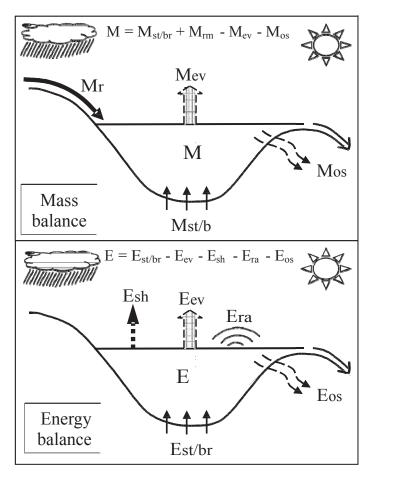
Figure 2. The diagram of mass and energy balance for a crater lake.
