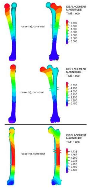
Figure 3: Displacement distribution on the bone-implant construct under walking loads for three boundary and loading cases in the medial (left) and anterior (right) views. Top: case (a), middle: case (b), and bottom: case (c). Displacements are exaggerated 10x for clarity.
