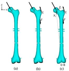
Figure 2: Boundary and loading conditions considered in this study: Case (a) consists of hip contact force with fixed boundary conditions on the distal condyles. Case (b) is the same as (a), including additional musle forces (abductor, tensor fascia latae and vastus lateralis). Case (c) corresponds to pyhsiological conditions with joint constraints.
