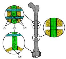
Figure 1: Meshed view of the bone-implant construct with section views of the contact regions, i.e., b/p: bone to pin, n/p: nail to pin and b/n: bone to nail.
