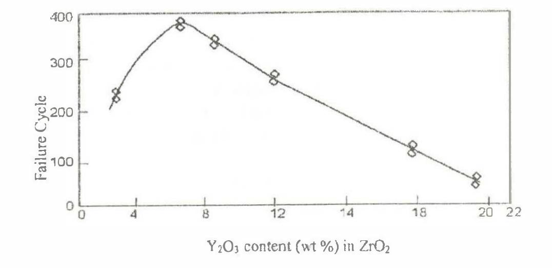
Figure 1. The effect of  $Y_2O_3$  Content (wt %) in  $ZrO_2$  on TBC life (16).
