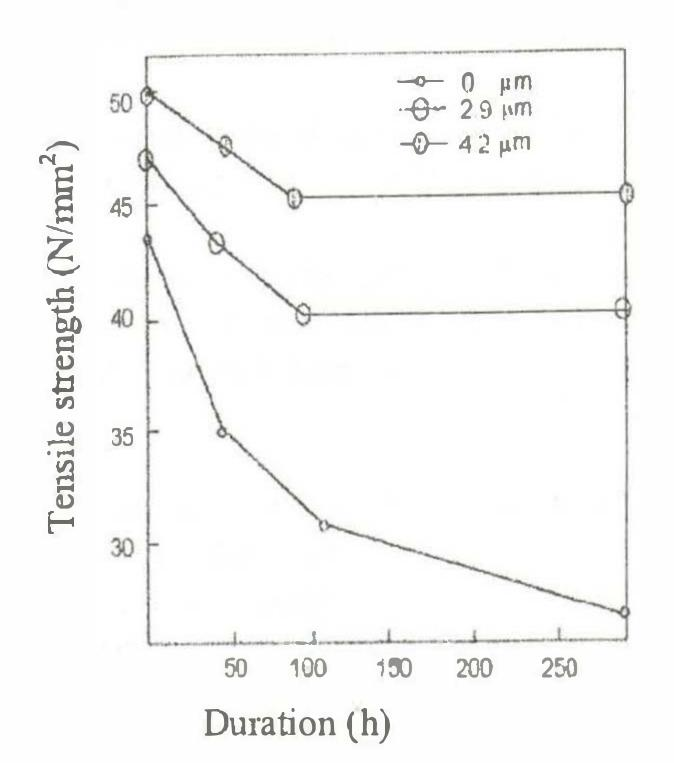
Figure 5. Tensile strength variation at the interface between top coat and bond coat after 10 thermal shock cycles [21]
