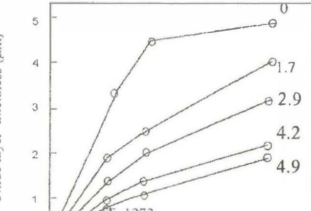
Figure 4. Variations of oxide layer thicness with respect to diffusion barrier coating thicness at 1273 K and 1373 K. The bond coat composition is Co-31Ni-21Cr-8Al-0.5Y(21)
