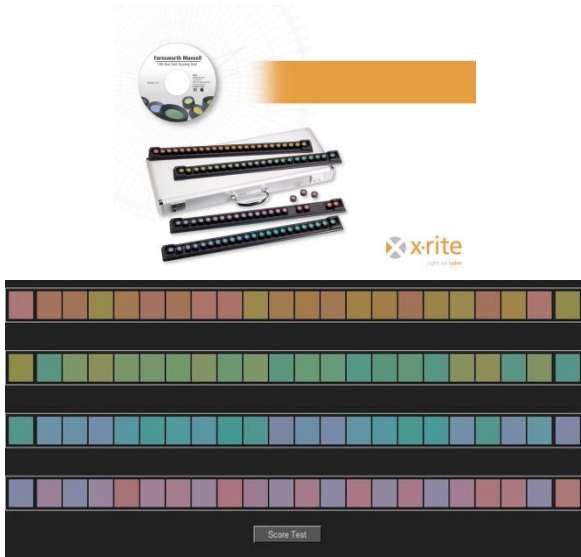
Fig 1: Farnsworth munsell 100 hue test Manual apparatus (above) and software based system on (below)
