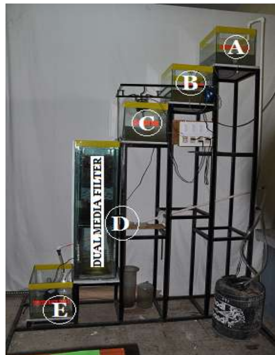
Fig. 1: Experimental set up of Lab scale wastewater treatment plant, (a) Sedimentation (b) aeration (c) agitation (d) Filtration Unit and (e) collection tank.
