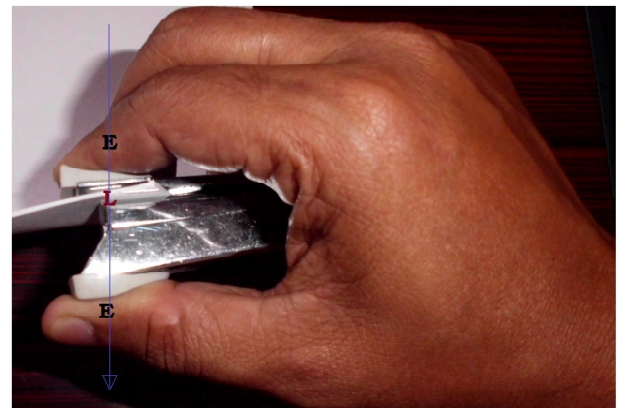
Photograph 5: The line joining load (L) and the points of efforts (E) looks perpendicularly intersecting the stapler.
