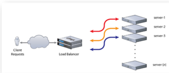
Fig. 1- load Balancing Architecture
