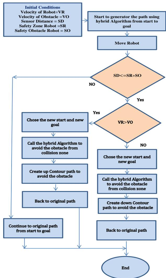
Figure.7 Proposed algorithm to make the robot avoid collision with the dynamic obstacle
