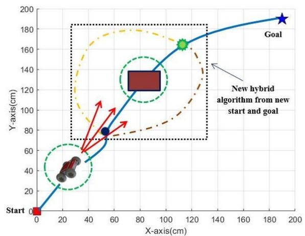
Figure. 11 Hybrid algorithm to avoid the obstacle from the collision zone
