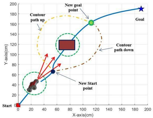
Figure. 10 Up and down contour path
