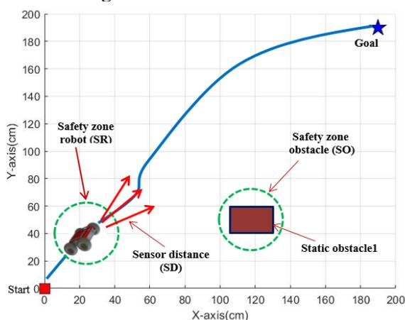
Figure. 5 Static environment with one static obstacle
