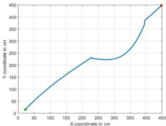
Figure. 25 Optimal path generated based on the proposed RRT\*PSO hybrid algorithm
