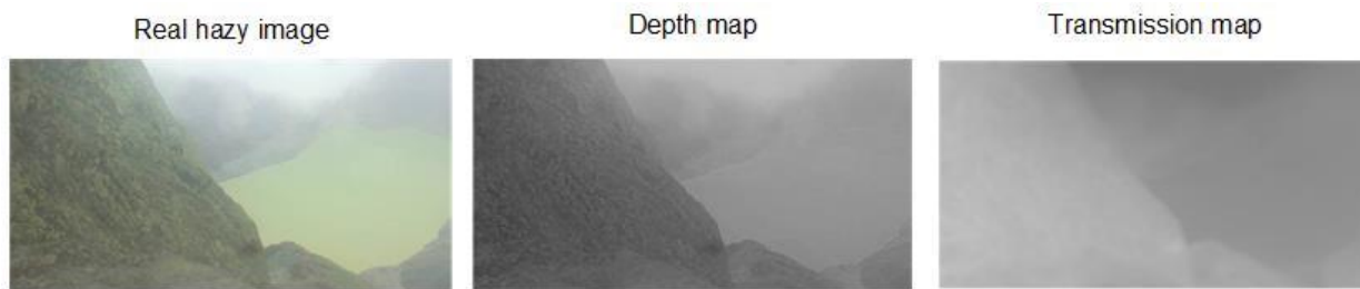
Figure. 3 The depth map and the transmission map for real hazy image at 03 Oct 2017 03:17 PM
