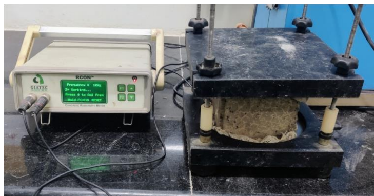
Fig. 3 Set up for measuring electrical resistivity of concrete
