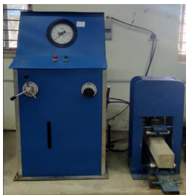
Fig. 2 Arrangement for flexural strength test for concrete beams
