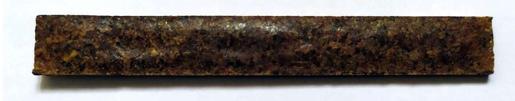
Fig. 2. Test sample of solid fuel from corn alcohol distillery stillage after pressing for 60 s (sample 1)
