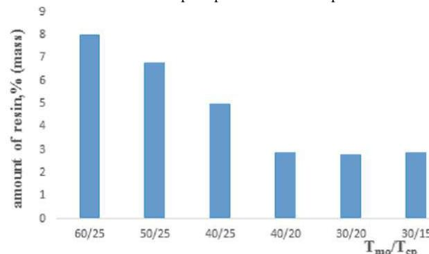
Fig. 4. The effect of model oil and «cold finger» temperature on the number of deposited asphaltenes
