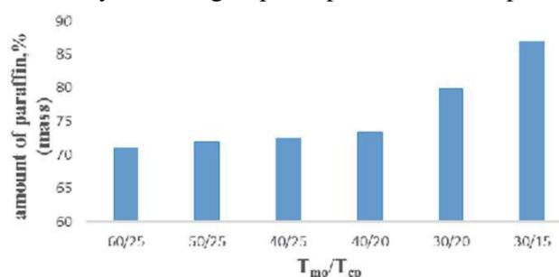
Fig. 2. The effect of model oil and «cold finger» temperature on the number of precipitated paraffin hydrocarbons
