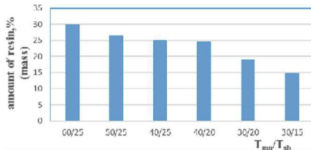
Fig. 3. The effect of model oil and «cold finger» temperature on the number of precipitated resin components
