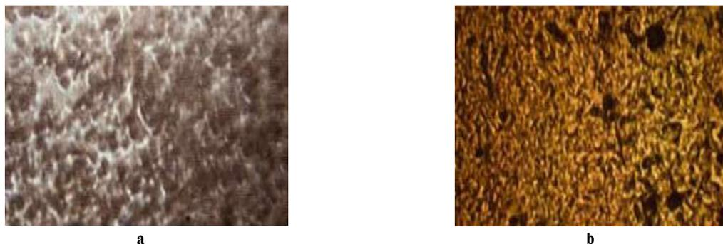
Fig. 11. Microphotography of model oil deposits with and without additives: a – model oil, b – model oil+«Difron-4201»
