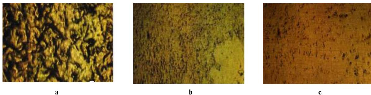
Fig. 6. Formation of paraffin hydrocarbon crystals in sediments separated at different temperatures of the model oil and «cold finger» (°C): a – 60/25, b – 40/20, and c – 30/15
