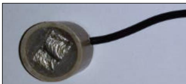
Figure 7. Weld overlay cladding samples for polarization test
