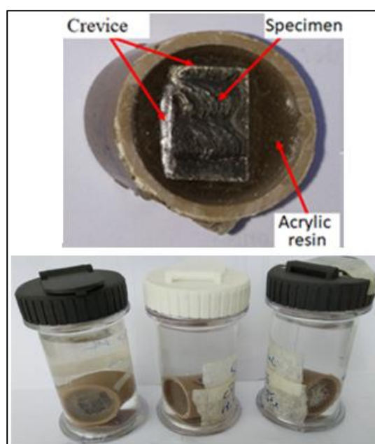
Figure 8. Samples used in the corrosion tests and immersing into a 100 mL acrylic container containing 3.5% wt. NaCl solution at 40 °C
