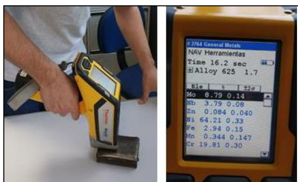
Figure 6. X-ray fluorescence (XRF) determination with the portable analyzer NITON XLT 898 on the overlay cladding samples
