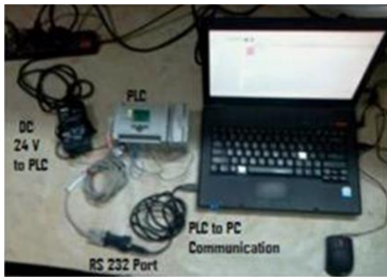
Figure 4. PLC to PC Communication.
