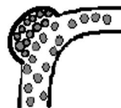
Figure 2. Using the grains to protect the pipe.
