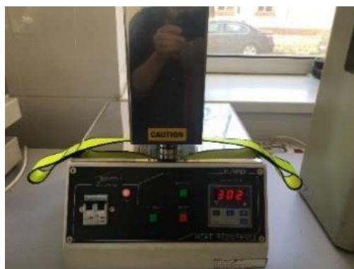
Figure 2 - Apparatus for testing the contact heat resistance
