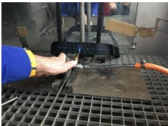
Figure 1 - Flame exposure system
