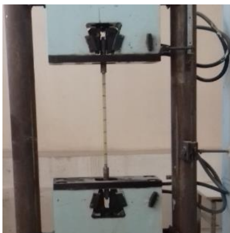
Figure 2. The process of elongation testing of a sample of glass composite reinforcement
