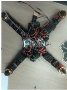
Figure. 2 The realized quadrotor
