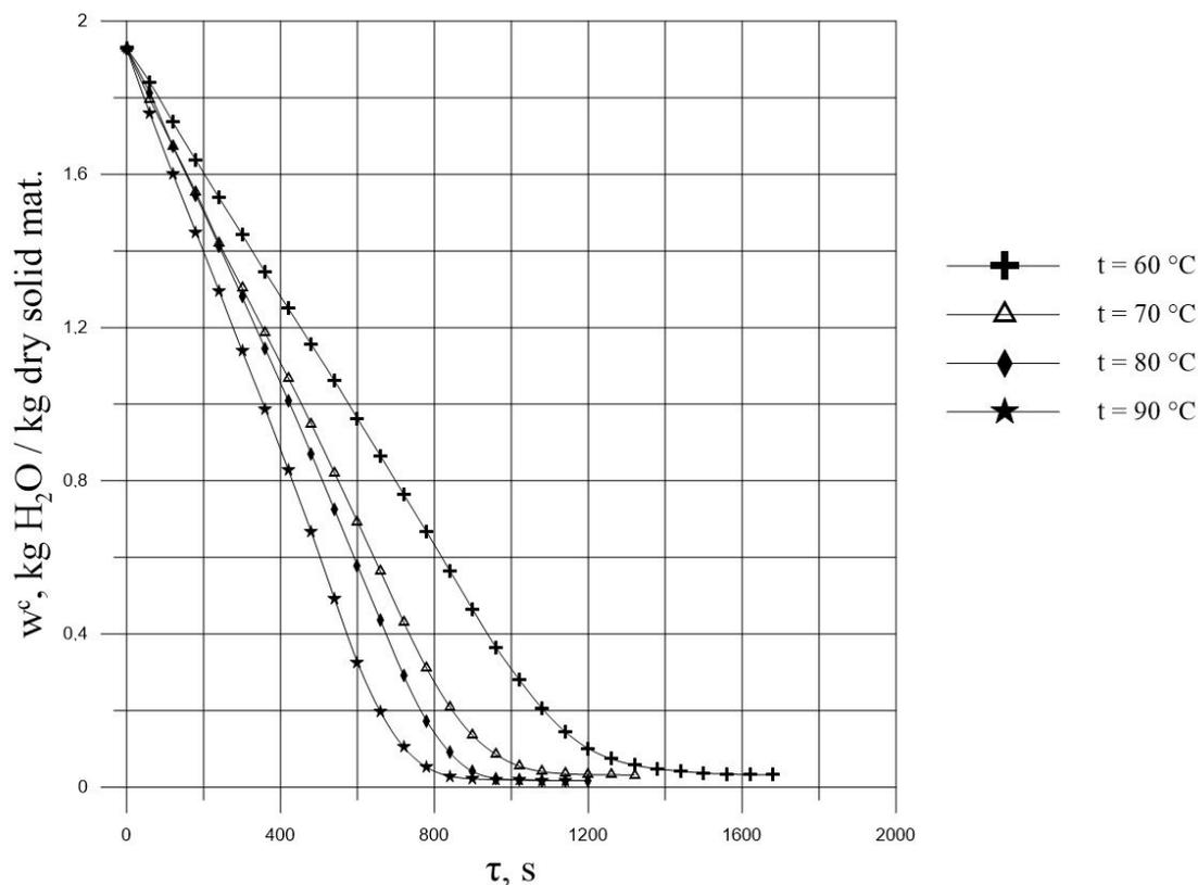
Fig. 3. Kinetics of filtration drying of corn distillery stillage at different temperatures of the heating agent ( $H=120$  mm)
