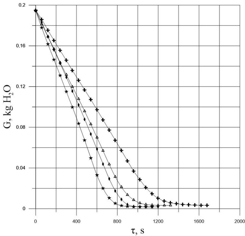
Fig. 5. Change in the moisture mass of corn distillery stillage as a function of time at different temperatures of the drying agent at a layer height  $H=120$  mm
