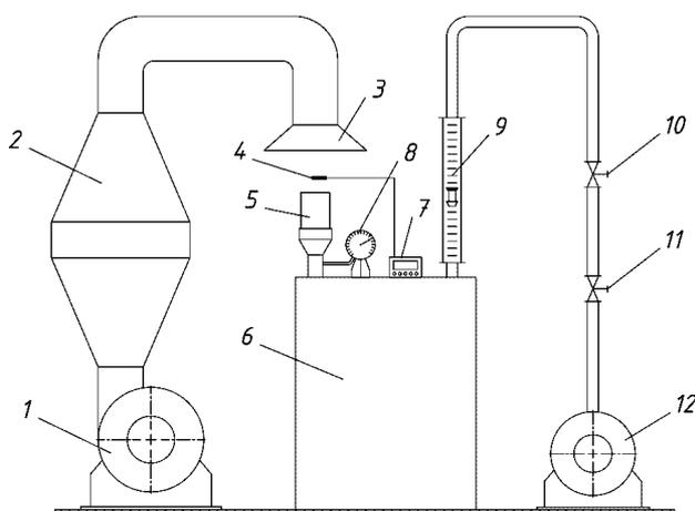
Fig. 1. The scheme of the experimental installation for filtration drying: 1 – fan; 2 – electric heater; 3 – diffuser; 4 – thermocouple; 5 – container; 6 – receiver; 7 – control and measuring device SENTOS D1S; 8 – vacuum gauge; 9 – rotameter; 10 – control valve; 11 – shut-off valve; 12 – water ring vacuum pump
