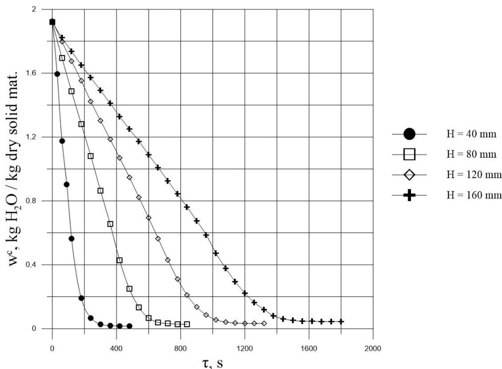
Fig. 2. Kinetics of filtration drying of corn distillery stillage at different layer heights ( $t=70^\circ\text{C}$ )
