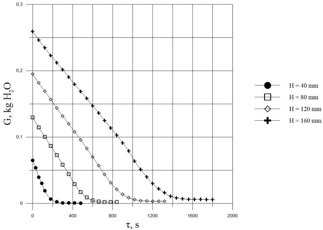
Fig. 4. The change in moisture mass of corn distillery stillage as a function of time at different layer heights at  $t=70^\circ C$
