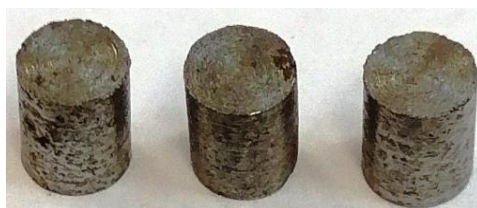
Figure 2 – The cast iron specimens for realization of compression testing.
