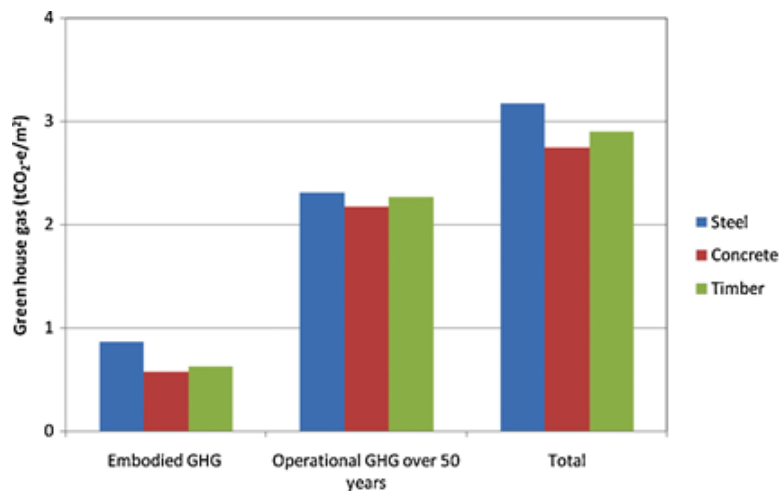
Fig. 6. GHG emissions of the three featured construction materials of eight-storey multi residential building (Aye et al., 2012).
