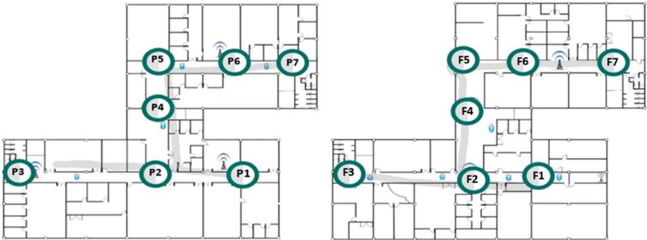
Figure. 3 Assigned position and the recorded path testing at the second floor (left) and third floor (right)
