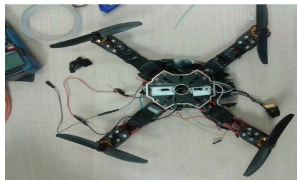
Figure. 7 Top view of the realized quadcopter
