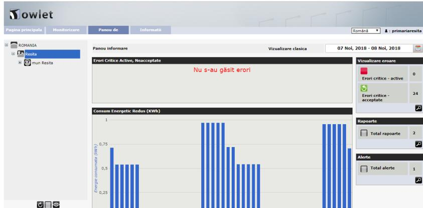
**Figure 5.** Electricity consumed by a luminaire and dimming in the period 7-8 November, 2018.
