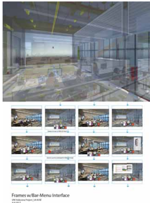
Figure 5. (a) Simulated view- HoloLens™ showing projection of Revit model on top of actual physical space, (b) Frames with bar menu interface.
