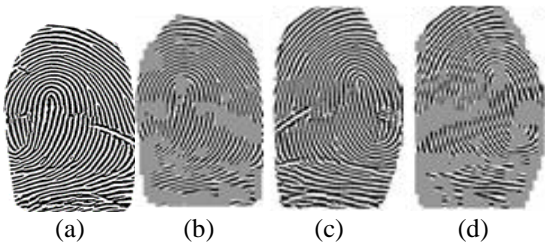
Figure. 5 The quality assessment and classification: (a) the original fingerprint, (b) results of classification by the coherence, and (c) results of classification by the variance, where the red, green, blue and black represent high, medium, low and bad quality types respectively
