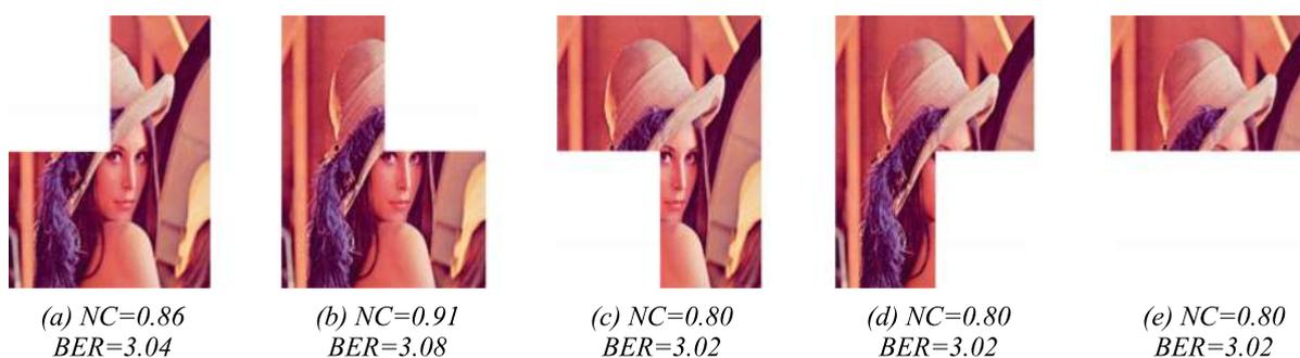
FIG. 6. WATERMARKED “LENA” IMAGE WITH NC AND BER VALUES AFTER PERCENTAGE CROPPING
