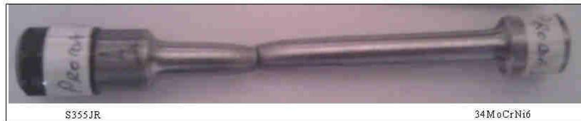
**Figure 5.** Sample no. 1 after the traction testing
