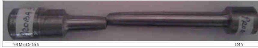
**Figure 7.** Sample no. 5 after the traction testing
