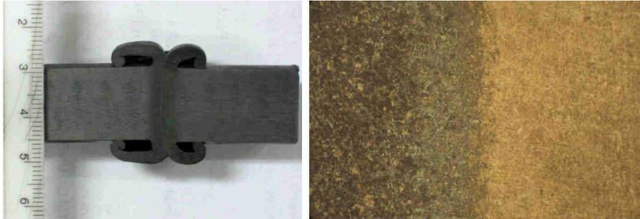
**Figure 10.** Sample no. 6: Macrostructure and shrunk area, 100x
