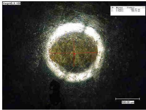
Figure 7. Micrograph of the 100Cr6 ball wear track against CuAl10Fe3.
