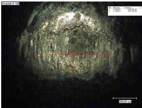
Figure 8. Micrograph of the 100Cr6 ball wear track against AlSi12.
