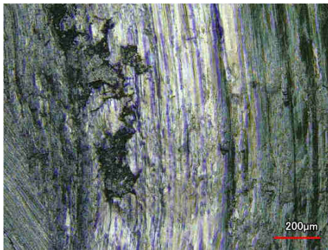
Figure 11. Micrograph of the sliding wear track for AlSi12 sample.
