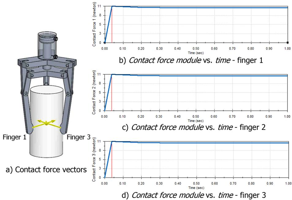
**Figure 6.** Determination of contact forces between gripper fingers and workpiece.
