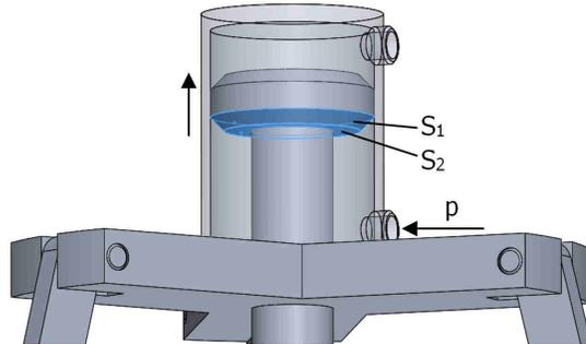
**Figure 4.** Gripper's pneumatic cylinder.
