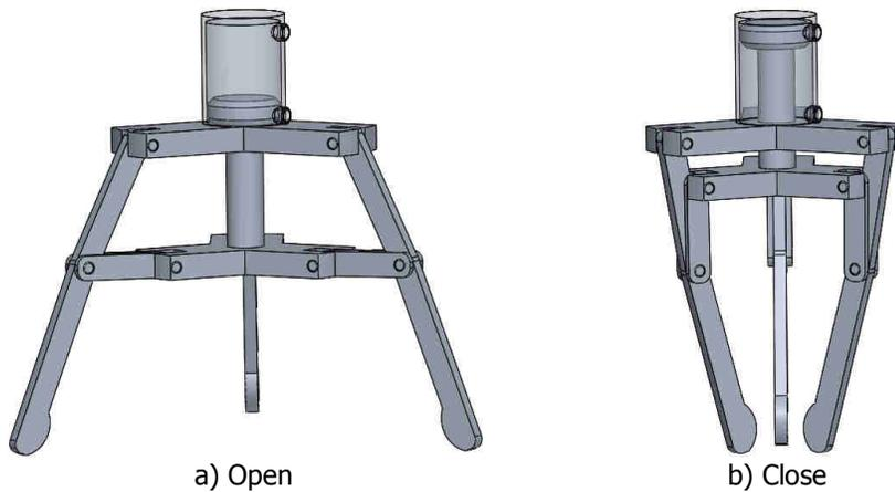
**Figure 2.** Positions of the robotic gripper model.
