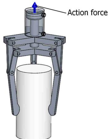
**Figure 5.** The action force applied on the piston.
