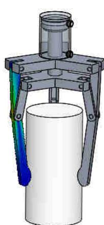
a) The finger in the gripper assembly
