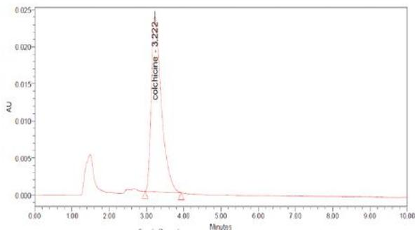
Fig 2: The Chromatogram showing the presence of Colchicine in Cell Culture Extract
