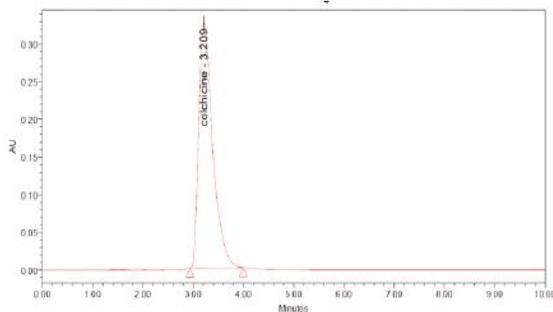
Fig 1: HPLC Chromatogram of Standard Colchicine
