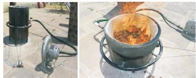
Fig. 1 Photograph of biomass combustion chamber with blower.
