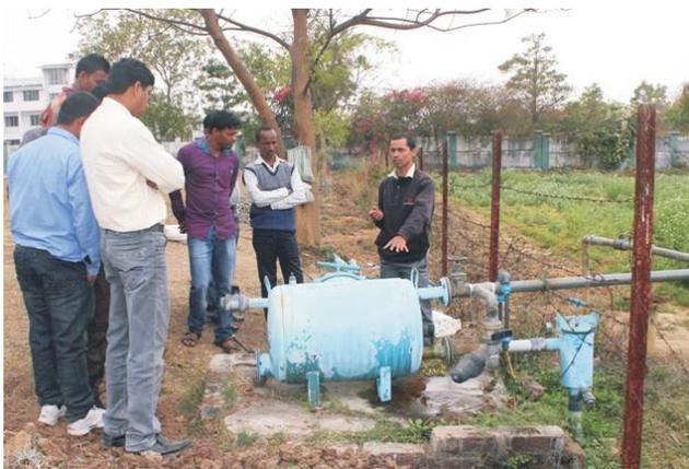
Fig. 6 : Drip irrigation with fertigation system.
