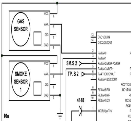
Fig 3: circuit of interfacing mq-6 as an lpg and smoke detector
