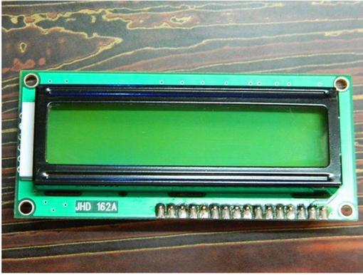
Fig 10: Liquid Crystal Display
