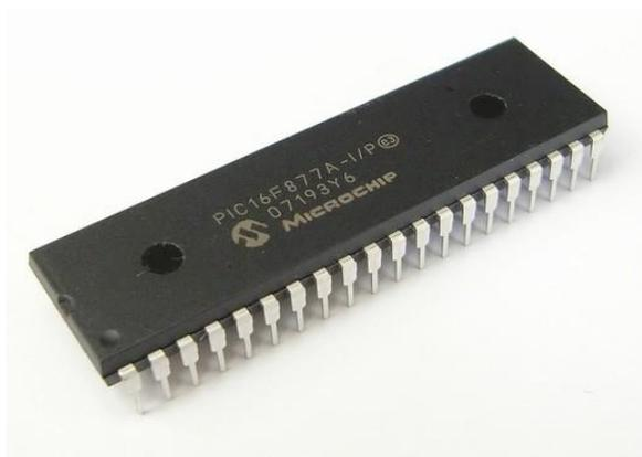
Fig 6: PIC16F877A Microcontroller
