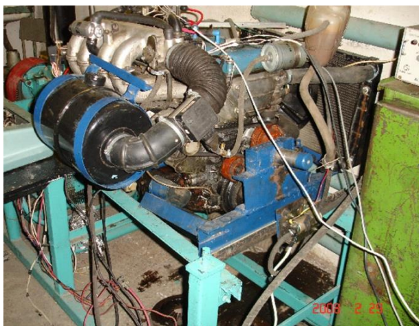
Fig. 9. Research stand for testing the ZMZ-4062 engine.
