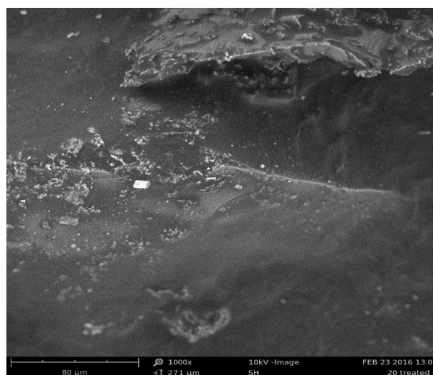
Fig. 9. SEM Image of the Fractured Treated Cow Hair Fiber Reinforced Composite.
