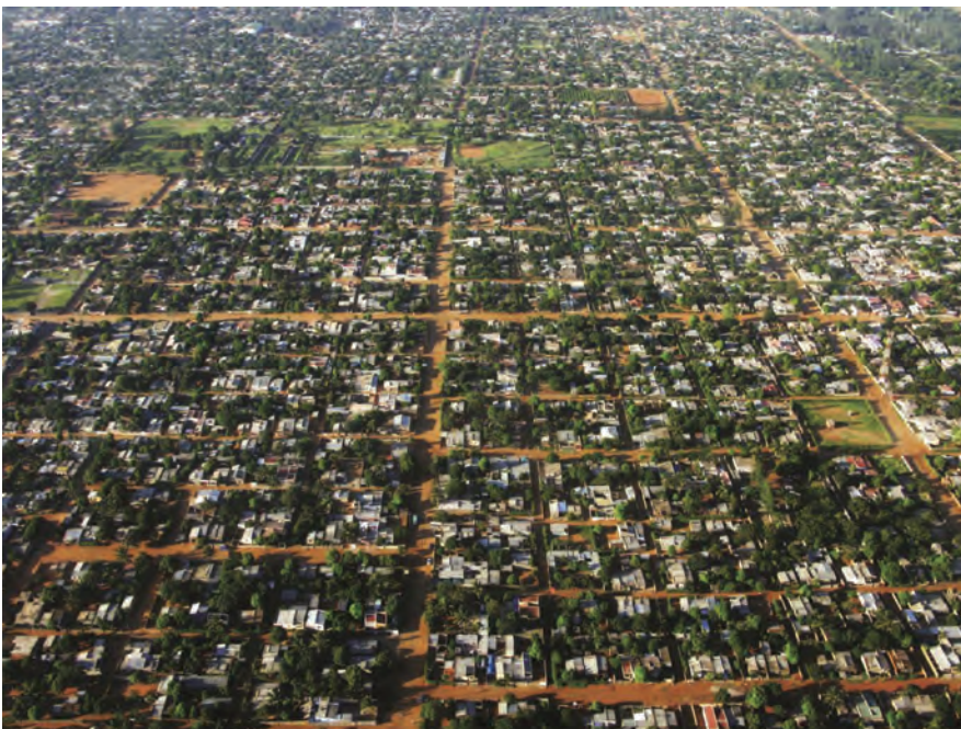
A planned suburban area with small plot sizes (12,5x25M) and some open spaces for recreation and other urban amenities. Planned in 1985 and implemented incrementally. Infrastructure provision is still rudimentary.
