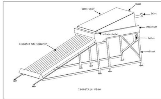
Figure 1 Solar Still Coupled With Evacuated Tube Collector
